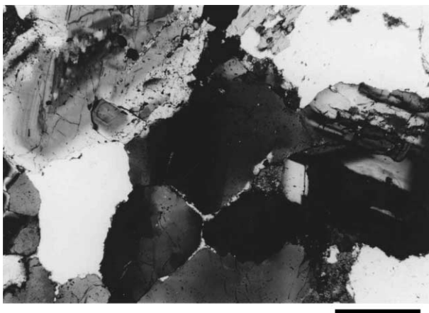
Fig. 2. Photomicrographs of the Kakkonda granite (core No. 12) from the borehole WD-1a. Undulatory extinction of quartz. Scale bar is 0.5 mm.
